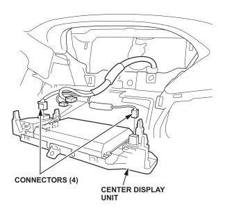
10. Locate the green 2-way transceiver connector secured to the vehicle harness. Remove the green tape to free the connector from the vehicle harness.
