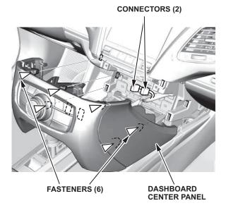
4. Remove the driver's inner dashboard trim and disconnect the connector.
