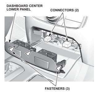
3. Remove the dashboard center panel and disconnect the connectors.
