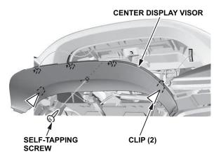
Remove the center display unit. Release the clips using the plastic trim tool and rotate the bottom of the display up slightly while pulling away from the opening.
