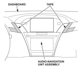
7. Pull out the audio-navigation unit assembly and disconnect the audio unit connectors.
