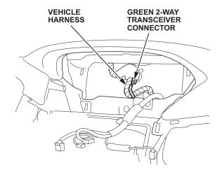
11. Slide the transceiver on the antenna bracket as shown.
