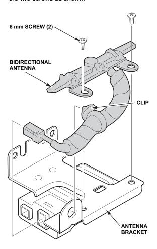
13. Plug the bidirectional antenna into the transceiver and secure the clip on the harness to the bracket.
